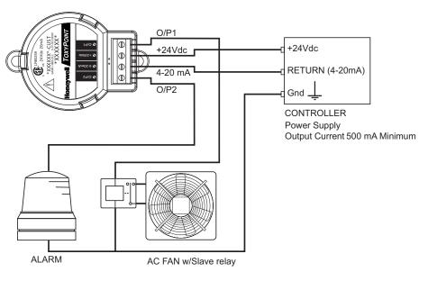
Alarm Outputs: Not to exceed 250mA @ 24VDC
