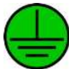
Figure 3. Protective Earth (Ground) Point
