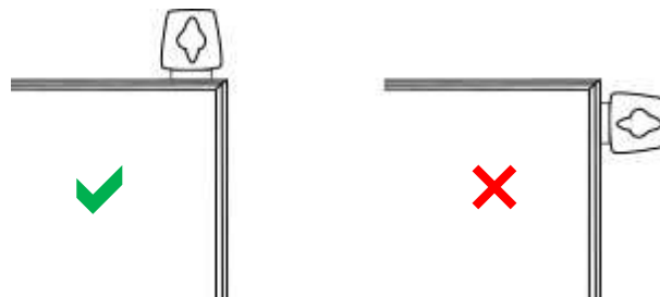
Figure 31. TPPER Correct Enclosure Mounting Orientation
