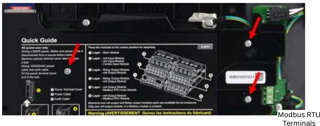
Figure 39. PCB Cover Screws (Arrowed)
