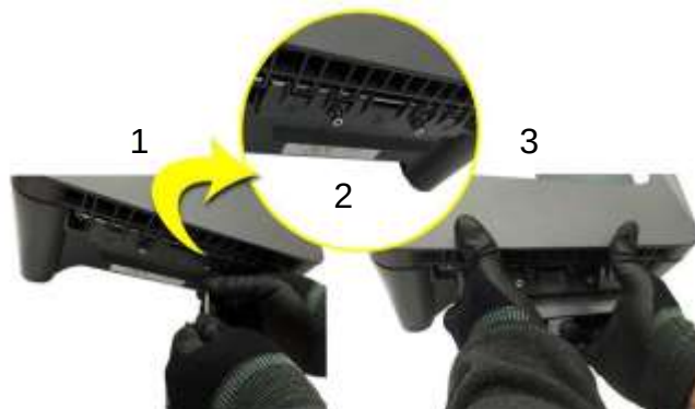
Figure 9. Undoing the Two Security Screws and Opening the Enclosure
