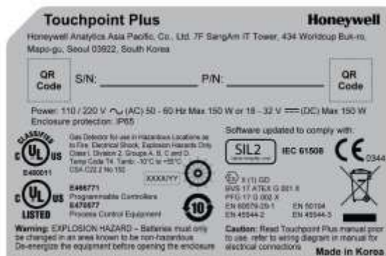
Figure 2. Rating Label (External – Not Shown Below)
