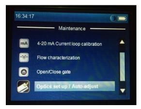
3. Remove Chemcassette Tape. Insert Optics Card – White Chip. Select Continue.
