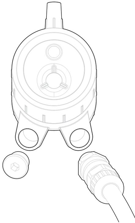
Figure 14. Connect cable glands to the Detector
