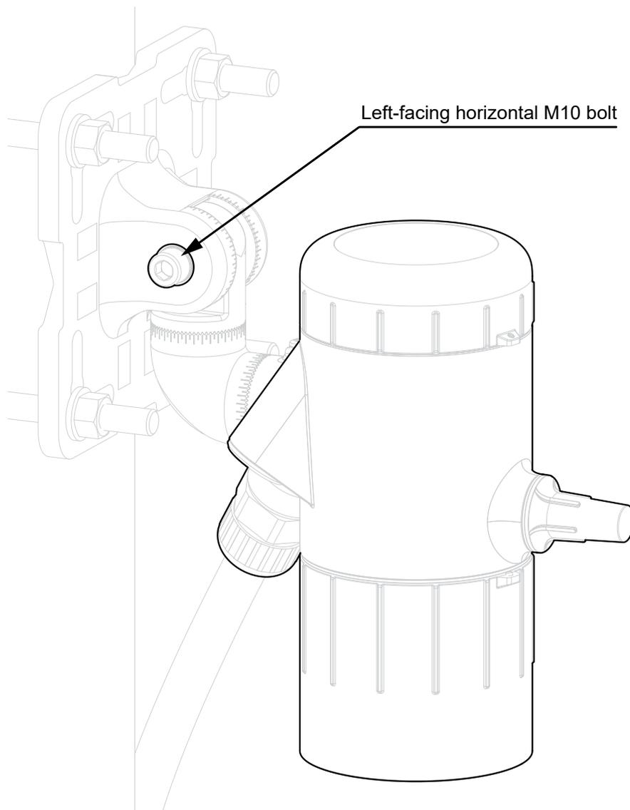
Figure 16. Set the vertical position of Detector to 0°
