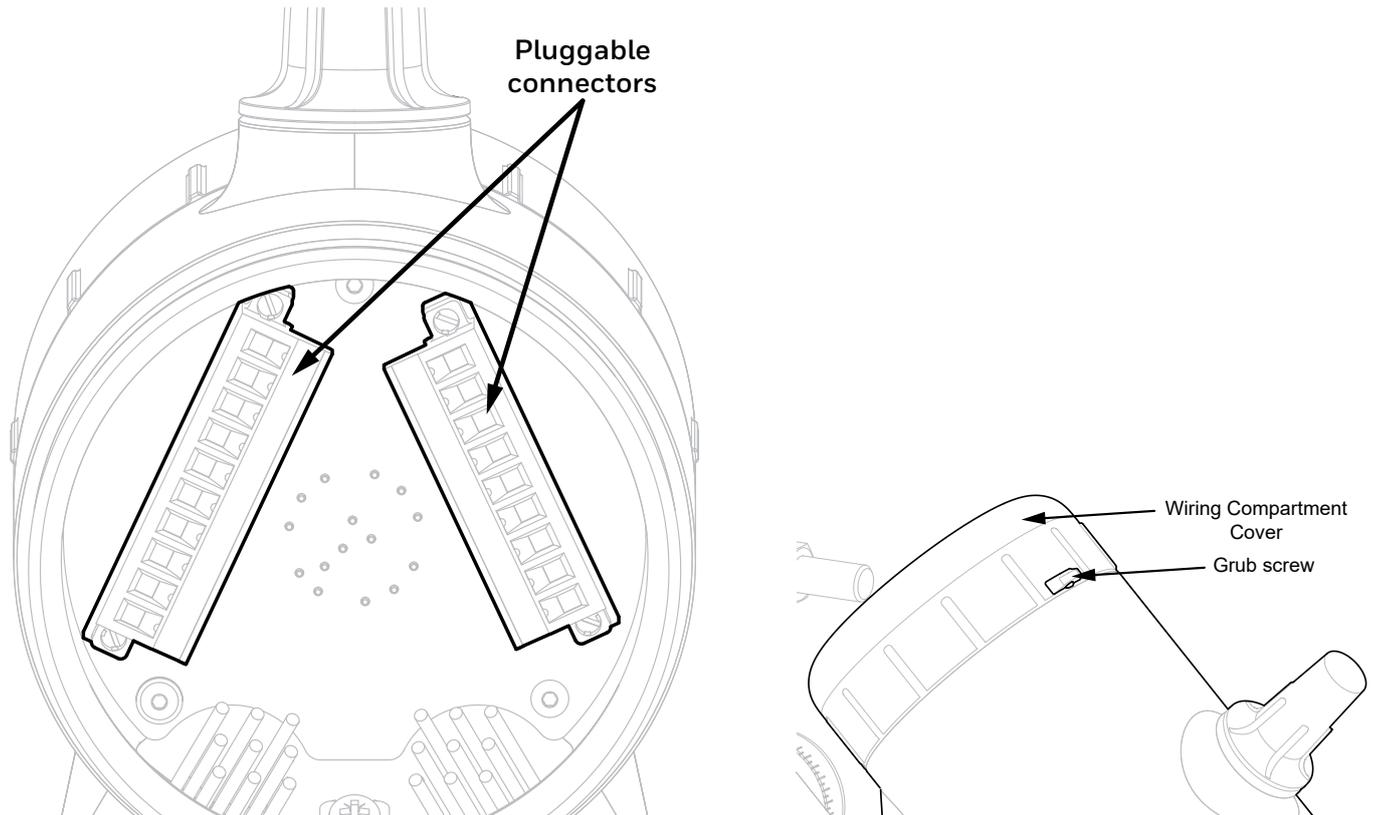
Figure 17. PCB Terminals
