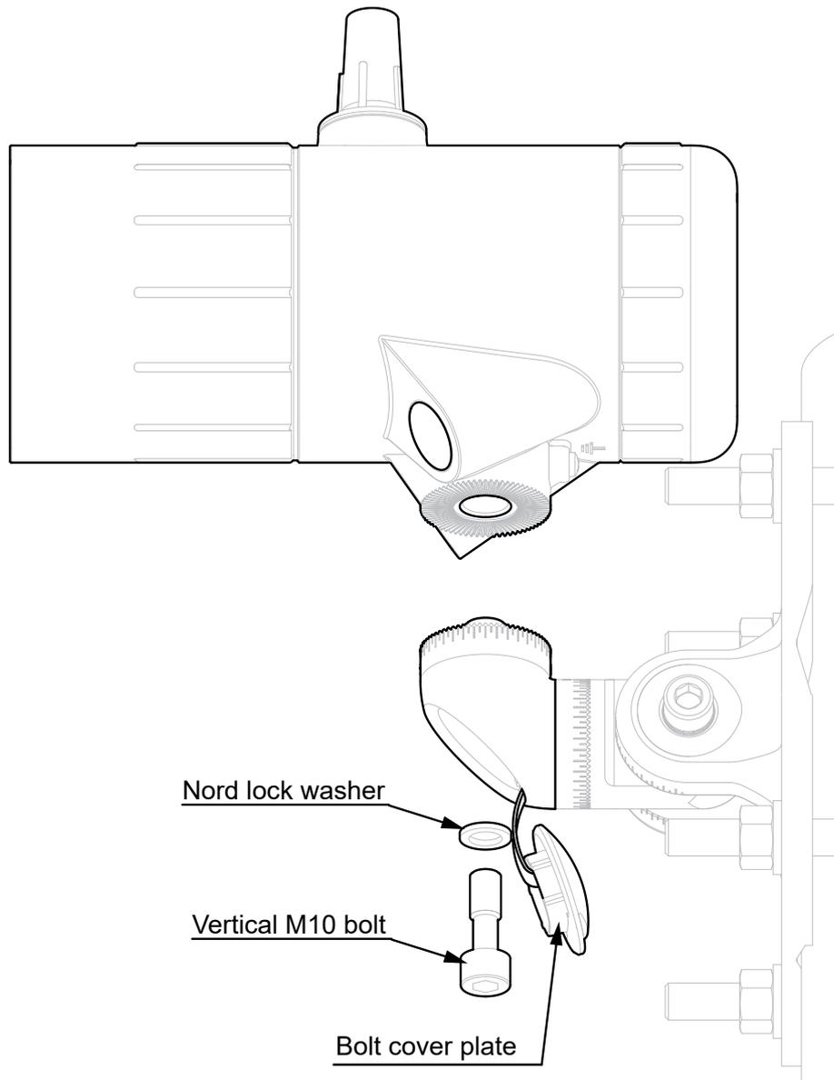
Figure 15. Detector attachment
