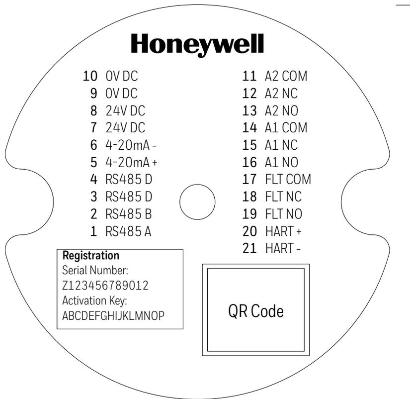
Figure 20. Terminal Connector Label
