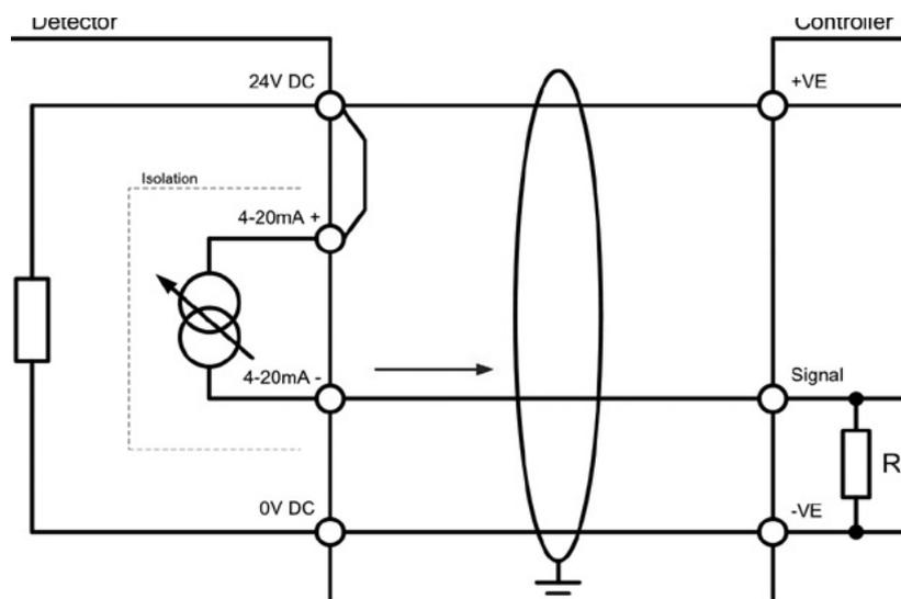
Figure 22. mA loop configuration as current source
