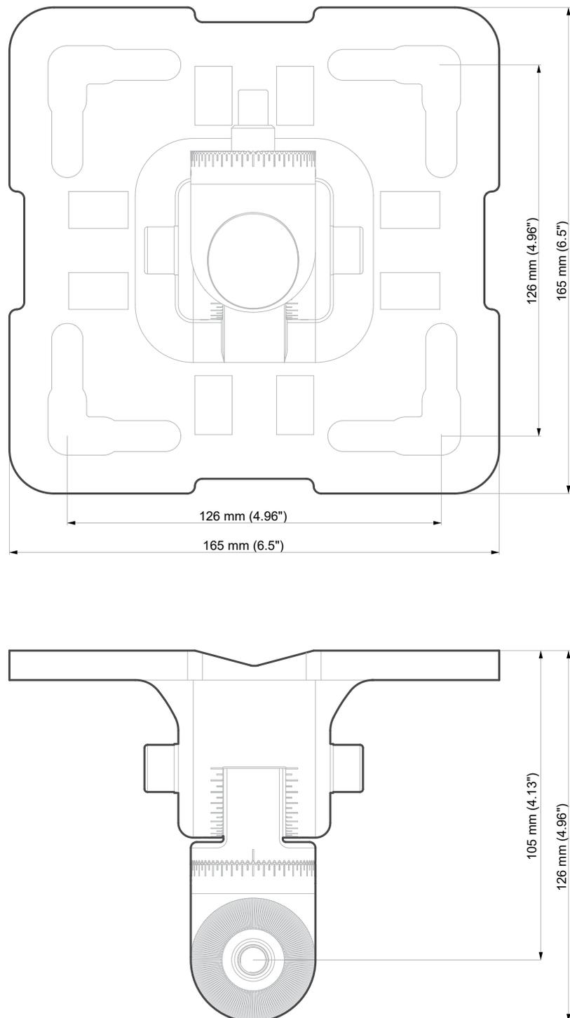
Figure 7. Universal Mounting Bracket general view and dimensions
