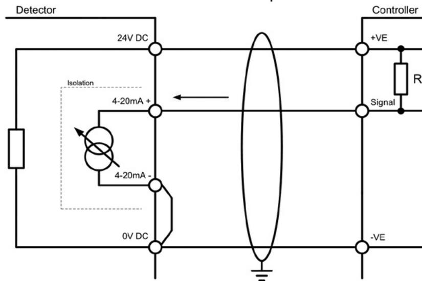
Figure 23. mA loop configuration as current sink
