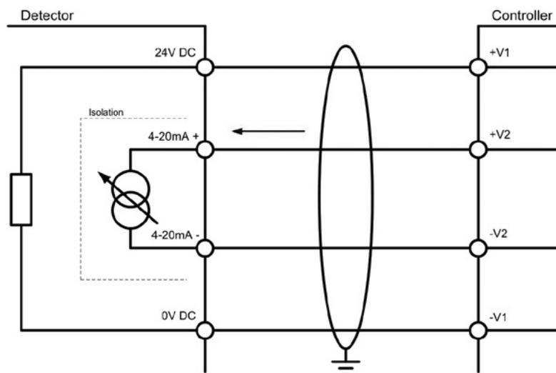
Figure 24. mA loop configuration as isolated output
