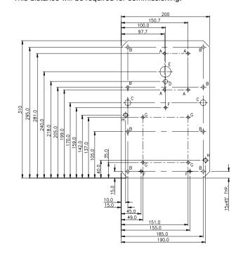
Insert the two mounting plate support bars through the aperture and attach them to the inside of the duct using M6 washers and nuts. Ensure that the threaded holes in the support bars line up with the holes drilled in the duct.
