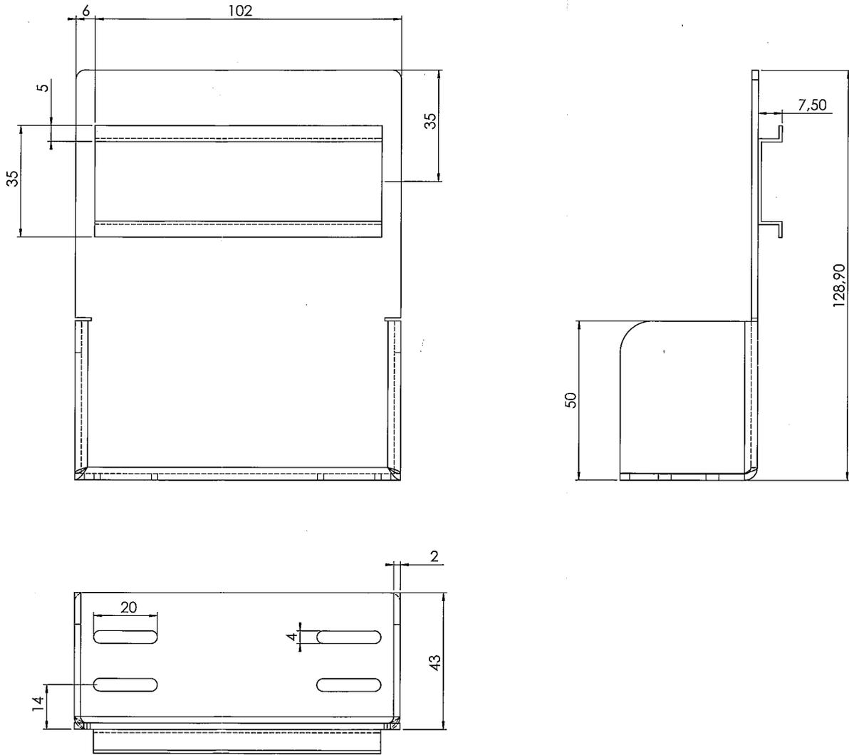
Optional L-shaped mounting plate with DIN-rail (P/N 9602.0051.10.02)
