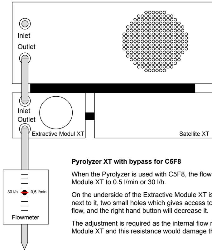
**Pyrolyzer XT with bypass for C5F8**
