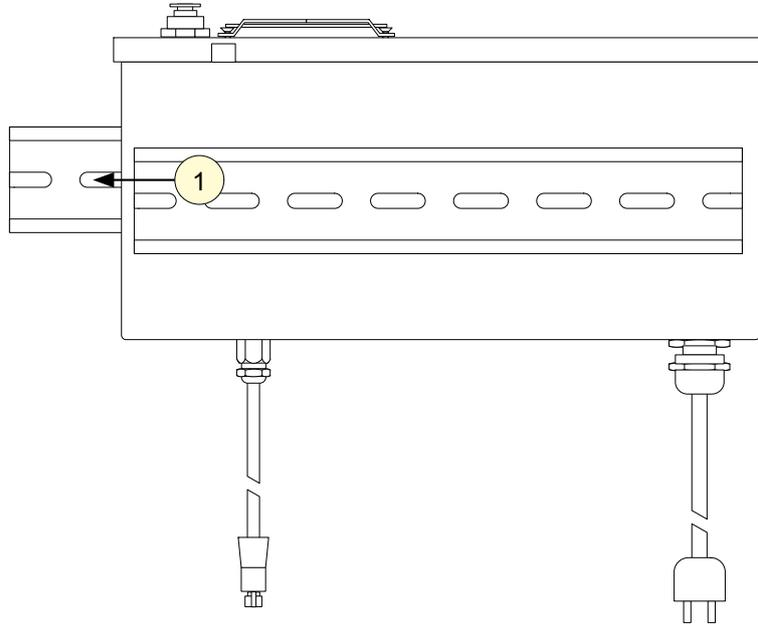
2. Slide the Extractive Module XT onto the rail at the front of the Pyrolyzer Module XT, see Figure 5.
