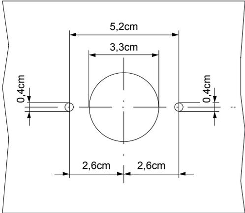
\*) Duct Mounting Saddle Assembly various types available, see spare parts list, Section 8, Reference Information
