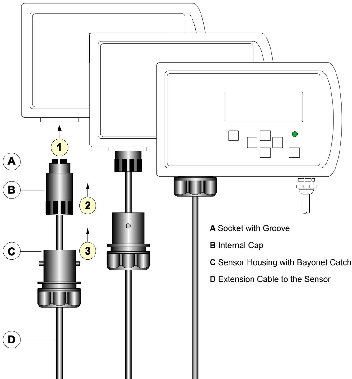
2.3.2 Mounting the Sensor Extension to the Duct
