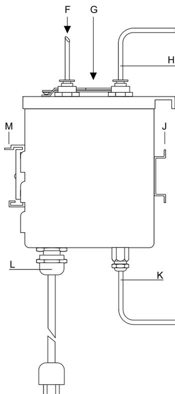
Figure 2: Front view of the complete assembly Pyrolyzer Module, Extractive Module, and Satellite XT.
