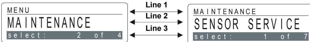
Line 1 shows the actual position in the menu. In the left example the actual position is Main Menu, in the right example it is the Sub-Menu Maintenance.
