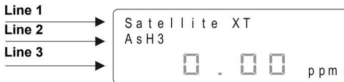
Depending on the operating mode the structure of the graphic display is different. Three basic versions are illustrated and explained below. A detailed description is given in the according sections.
