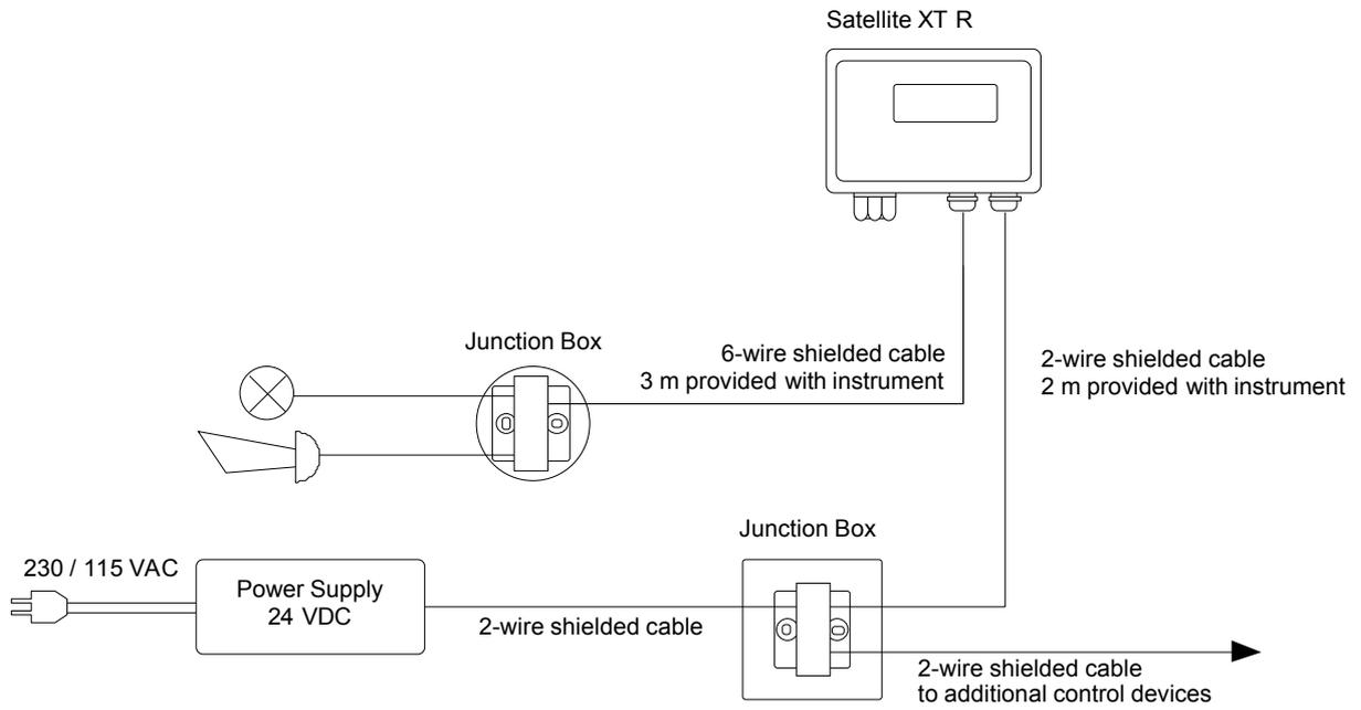
Wiring Diagram Satellite XT R - Basic Configuration
