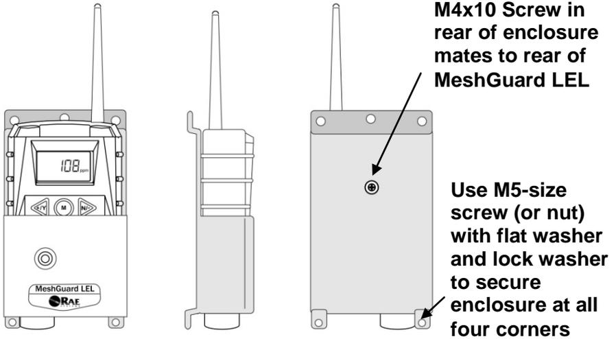
**Front, side, and rear views of the steel enclosure show how the MeshGuard LEL is secured for mounting.**
