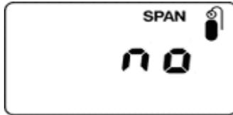
If the sensor fails, try to calibrate it again. If calibration fails again, replace the sensor.
