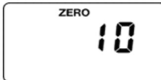
After the countdown reaches 0, the LCD displays “dn,” for “done.” The reading should show 0 (zero). Otherwise, repeat the zero calibration.
