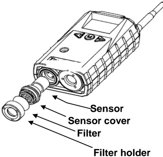
2. Use the hexagonal end of the tool to open the remove the sensor cover, turning counterclockwise.
