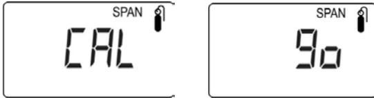
To start calibration, press [Y/+]. The LCD displays “go.”
