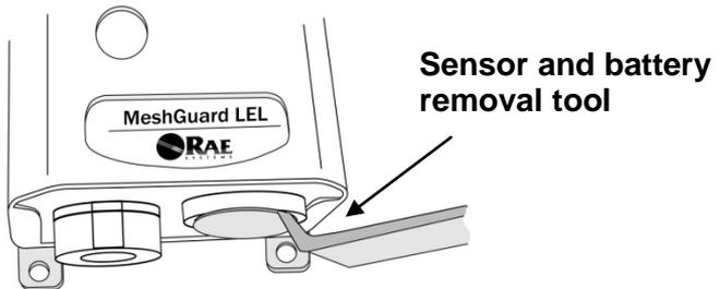
**WARNING:** Use only provided by Honeywell Analytics battery for the internal battery. If you need support with the p/n, please contact your Honeywell Analytics Representative. The internal battery must be replaced under a Hot Work Permit, where the atmosphere is determined to be non-hazardous while the battery is being replaced.
