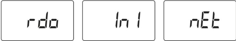
Note: If MeshGuard LEL is unable to find a radio network to connect with, it searches, and the display alternates between “rdo” and “Srh” (for “radio search”).
