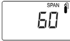
After counting down and reaching 0, the LCD displays “dn.” The reading should be the span concentration value. Otherwise, the span calibration should be repeated.
