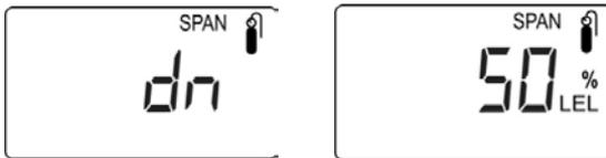
If the MeshGuard LEL does not detect gas after counting down to 0, the LCD displays “Err” (for “error”). The LED glows red and the buzzer sounds to provide extra warning. The MeshGuard LEL automatically returns to the span calibration display.
