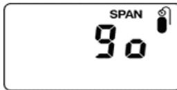
The MeshGuard LEL waits for 10 seconds so that you have time to connect the span gas. Connect the calibration gas adapter to the MeshGuard LEL, and connect the gas cylinder to the adapter. Start the flow of gas.
