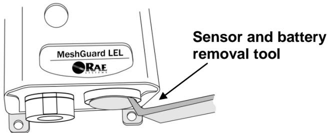
**WARNING:** Use only battery provided by Honeywell Analytics for the internal battery. The internal battery must be replaced under a Hot Work Permit, where the atmosphere is determined to be non-hazardous while the battery is being replaced.
