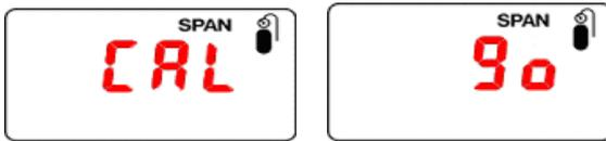
To start calibration, press [Y/+]. The LCD displays “go.”
