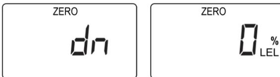
**Note:** When performing Zero Calibration, always make sure you do so in an environment with clean air.
