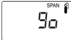
The MeshGuard LEL waits for 10 seconds so that you have time to connect the span gas. Connect the calibration gas adapter to the MeshGuard LEL, and connect the gas cylinder to the adapter. Start the flow of gas.
