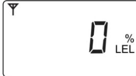
If the MeshGuard LEL finds and joins a wireless network, an antenna icon is shown in the display. If no link or a weak link is established, no antenna icon is shown. Press [Y/+] to manually search for a network.
