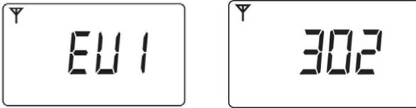
Press [MODE], and it alternates between Pan and ID (Personal Area Network Identifier) and its value (all units in a network must have the same Pan ID):
