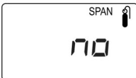
If the sensor fails, try to recalibrate it again. If calibration fails again, replace the sensor.
