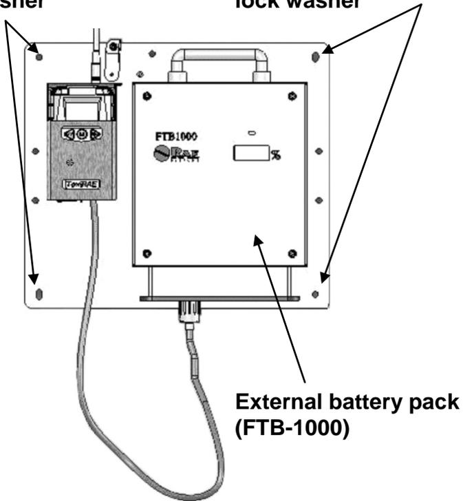
**Note:** The plate holding the battery pack and FTD-3000 LEL must be mounted on a solid, flat surface.
