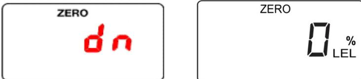
**Note:** To stop zero calibration before the countdown reaches 0, press any key. The LCD displays “no” and advances to the next programming menu, Span calibration.
