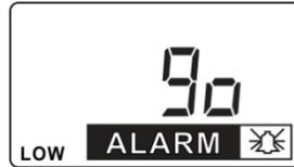
Press [Y/+] to enter and change the setting. Press [MODE] to exit and return to Detection Mode or [N] to advance to the next menu.
