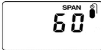
After counting down and reaching 0, the LCD displays “dn.” The reading should be the span concentration value. Otherwise, the span calibration should be repeated.
