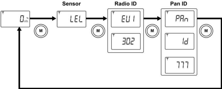
Press [MODE], and it displays the sensor type:
