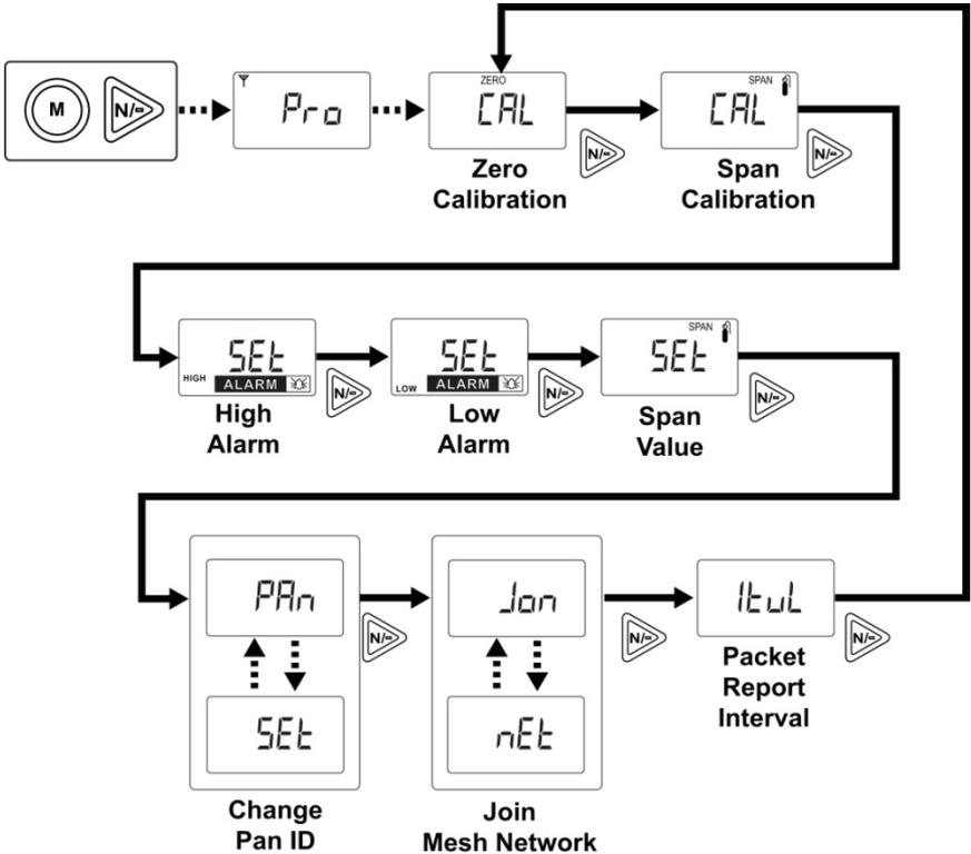
**Modify Span Gas Value.** This function allows selection of the gas concentration to the settings, press [MODE] to repeat stepping through the choices.
