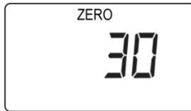
After the countdown reaches 0, the LCD displays “dn,” for “done.” The reading should show 0 (zero). Otherwise, repeat the zero calibration.
