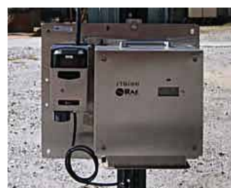
PowerPak connected to MeshGuard monitor. Monitor is shown in protective stainless-steel housing, secured with included hardware.
