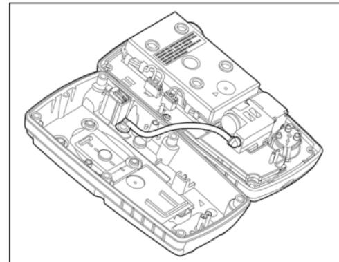
5. Remove the two PCB screws.
