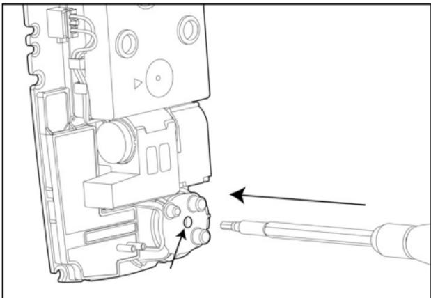
8. Insert the new sensor(s) and replace the sensor filter.
