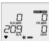
4. Refer to [Calibration and Bump Test Installation](#) (page 6). Attach the 0.5 l/min. regulator or the demand flow regulator and apply gas.
