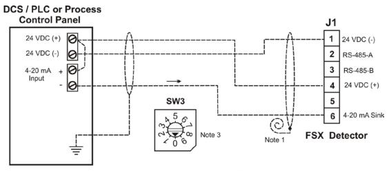
Non-Isolated 4-20mA (Sinking) Analog Output Wiring
