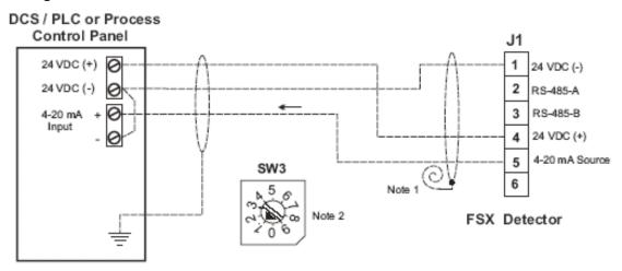
Non-Isolated 4-20mA (Sourcing) Analog Output Wiring
