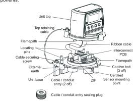
Width: 140mm Height: 150mm Depth: 152mm Height with Certified Sensor fitted: 270mm (282mm with O. sensor)
