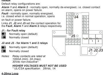
The table identifies the link and terminal connections for 4-20mA loop options
