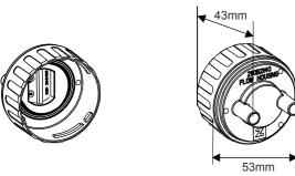
It can also be used in sampling systems where a sample of gas is drawn through a tube to the sensor. The accessory conforms to CSAC22.2 No. 152 when fitted to Certified Sensor with cartridge Part No: 2110B3754 installed.
