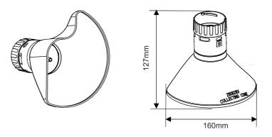
The Collecting Cone accessory is shaped to fit against a wall or other flat surfaces, and is designed to allow the gases collected to escape in a controlled manner so that the time to clear an alarm is not excessively prolonged.
