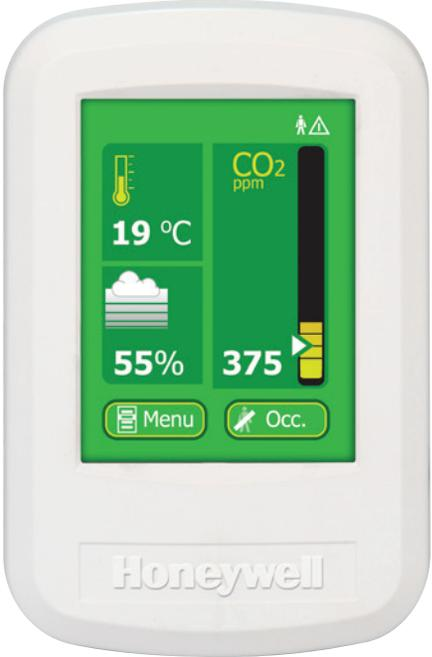
Improve indoor air quality and cut energy costs with CO<sub>2</sub> or VOC + temp/humidity monitoring for demand control ventilation. IAQPoint2 features a fully functional, multi-color, touch screen interface, the first of its kind. IAQPoint2 operates on +24 V<sub>AC</sub>/V<sub>DC</sub>. Analog output is 4-20 mA or 2-10 V<sub>DC</sub>, switch selectable. Digital output is BACnet/Modbus selectable or LonWorks. Available in wall mount and duct mount configurations.
