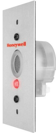
The ToxyPoint two wire transmitter provides continuous monitoring for carbon monoxide in ambient air and is designed to reduce the overall cost of ownership with a lower initial investment, eliminating maintenance costs and minimising building electrical operating costs. 2-Year disposable sensor, no calibration required.
