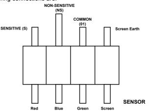
Following installation the sensor must be calibrated.
