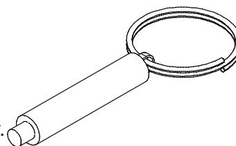
Hold the Magnetic Wand in position for up to 2 seconds = ●
