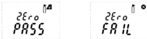
10. If using zero-air, turn it off. Zeroing is complete and saved.
