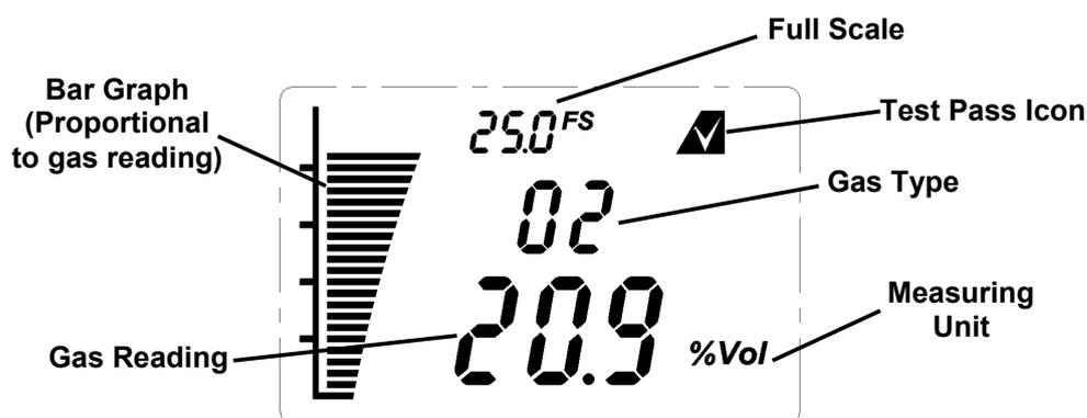
Diagram 12: Example of a O<sub>2</sub> Transmitter Display screen – Normal Operation
