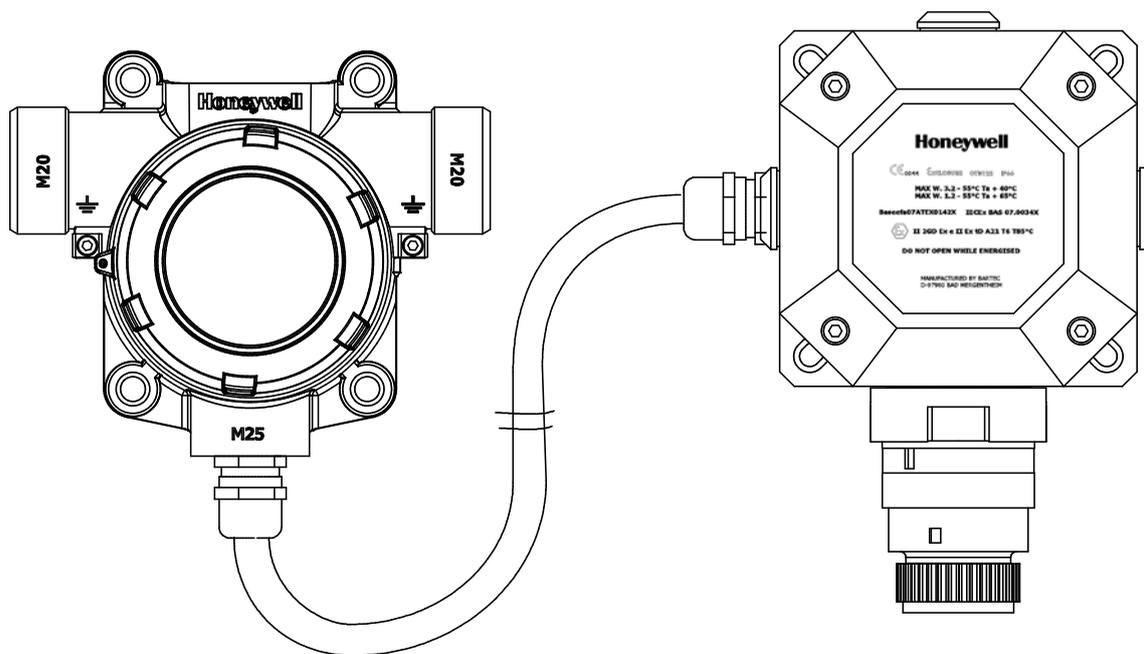
Diagram 7: Remote Sensor Mounting
