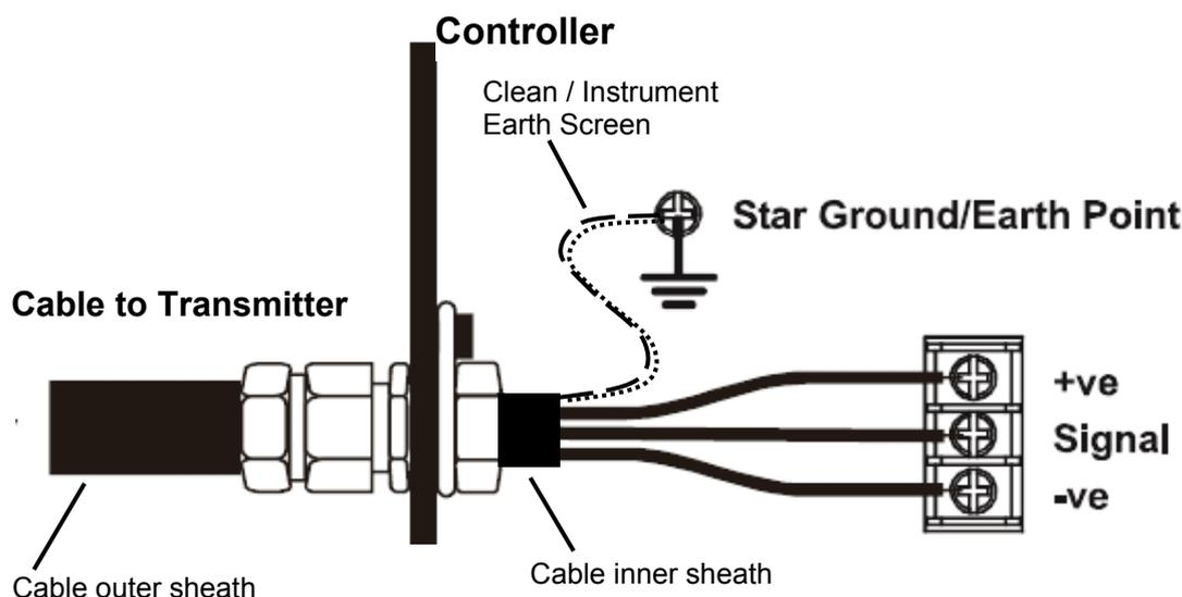
Diagram 10: Controller Grounding
