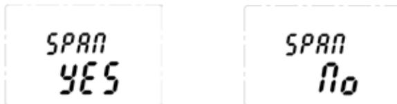
12. If span calibration is required use '✓' proceed to the next step. If span calibration is not required, use '▲▼' to select 'No' and '✓' to return to configuration mode.
