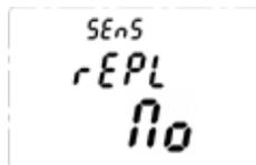
20. Use '▲▼' to select 'YES' if the sensor has been replaced or 'No' if it has not been replaced.
