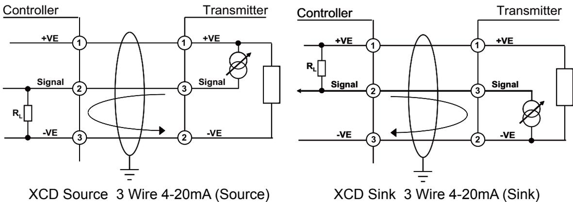
**Note: Terminate cable screen at transmitter or controller, not both. 250ohm load resistor (RL) is installed in the factory, In case of connection with controller, this resistor should be removed because controller has load resistor internally.**
