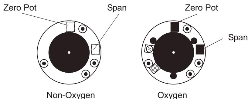
Diagram 15: Sensepoint Toxic Sensor Zero and Span potentiometer
