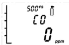
6. Observe the Zero reading on the XCD RTD display. If it shows a stable reading around "0" there is no need to carry out Hardware adjustment. Skip the next step.
