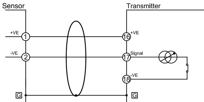
**Note: Ensure that the earth from the Sensepoint Toxic Sensor is connected to the Ground/Earth Point.**
