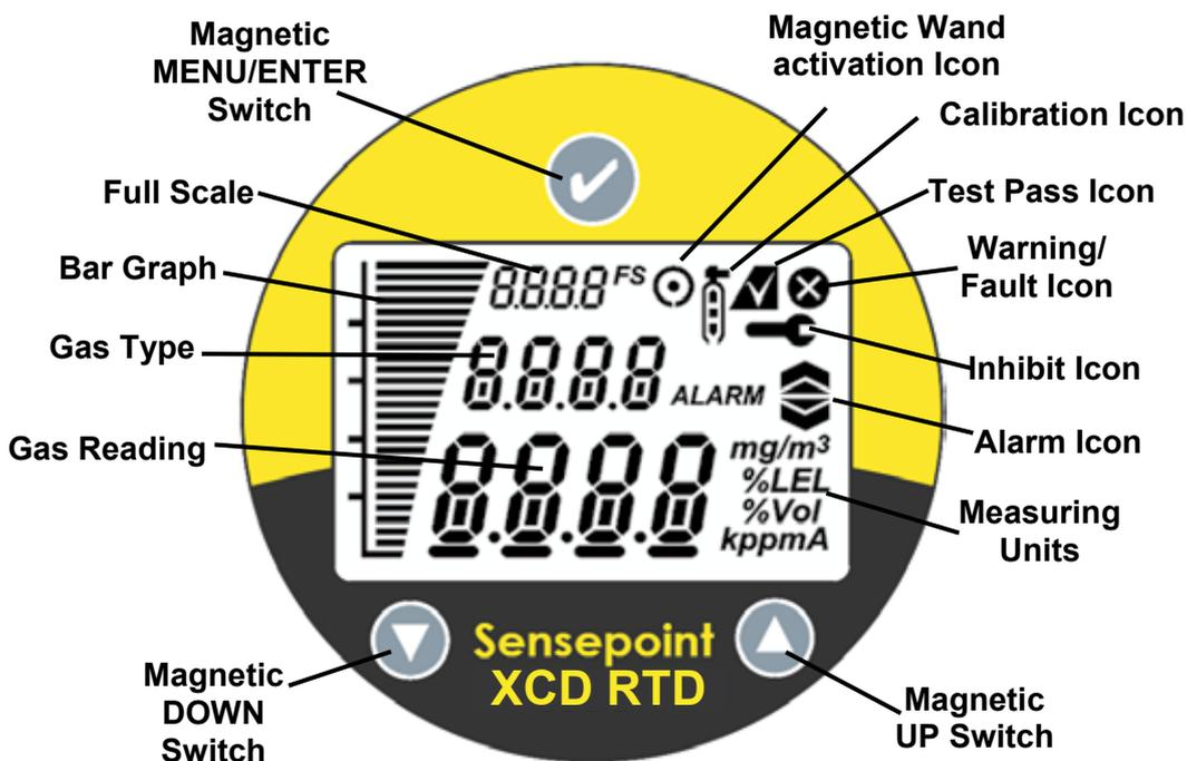
Diagram 2: Sensepoint XCD RTD Display and Magnetic Switches
