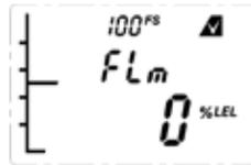
15. If the sensor has been replaced the following display may be shown.
