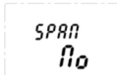
10. If span calibration is required use '✓' proceed to the next step. If span calibration is not required, use '▲▼' to select 'No' and '✓' to return to configuration mode.
