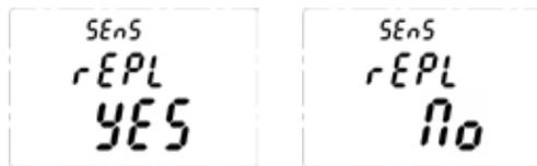
16. Use '▲▼' to select 'YES' if the sensor has been replaced or 'No' if it has not been replaced.
