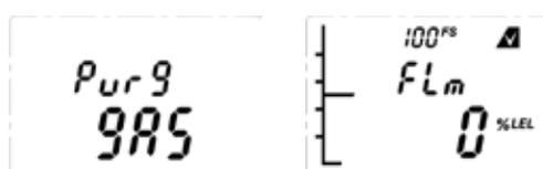
19. Promptly switch off the calibration span gas and remove the Sensepoint XCD Gassing Cap from the sensor to allow the gas to disperse.
