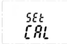
4. Put the magnet over the '✓' switch again and move to enter the Calibration menu.
