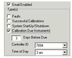
6. Directly beneath the "Calibration Due Instruments" checkbox are three controls that apply only to the calibration due reminder e-mails.
