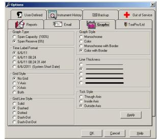
Setting the Graph Type to Span Reserve will shift the baseline of the graph to 0% on the graph. In this case, the observed span reserve will be indicated as a function of the 0% baseline. This means that if the sensor is healthy, it will have a positive span reserve value. Sensors showing a negative span value need to be replaced.
