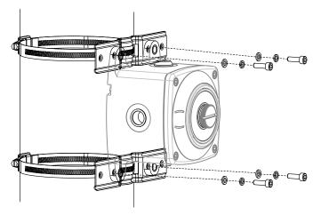
HALO may be fixed to a horizontal or vertical pipe of 50 to 150 mm (2 to 6 inches) in diameter using the optional Pipe Mounting Bracket.
