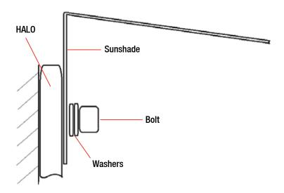
3. Ensure that the mounting bolts are fully re-tightened, using the long ball-end 5 mm hex wrench supplied with the sunshade.
