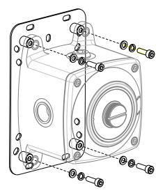
For retrofit applications, the optional adaptor plate kit enables HALO to be mounted in place of an existing DVC100 or Honeywell Analytics Junction Box. The plate has mounting holes corresponding to the hole centres of the DVC100 series and the Honeywell Analytics Junction Box.
