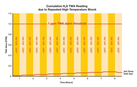
After repeated cycles of high temperature shock, measurable drift in the GasAlertQuattro did not exceed 0.1 ppm
